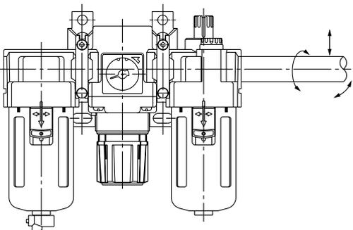
3. Piping materials without flexibility such as steel tube piping, are prone to be effected by excess moment load and vibration from the piping side. Use flexible tubing in between to avoid such an effect.
