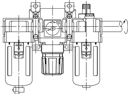
2. Avoid excessive torsional moment or bending moment other than those caused by the equipment's own weight as this can cause damage.
